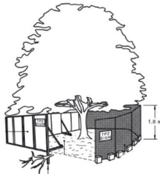
Figure 2: Indicative TPZ fencing
