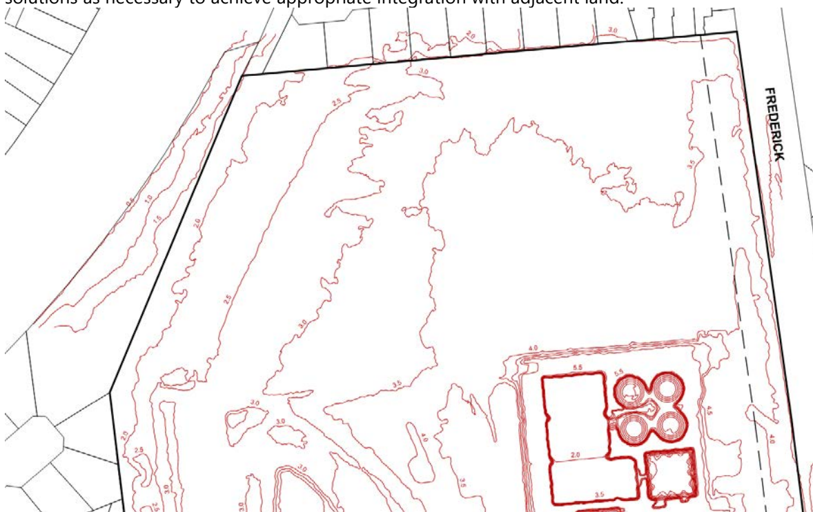
Figure 5 - Existing site levels in mAHD (LiDAR)
