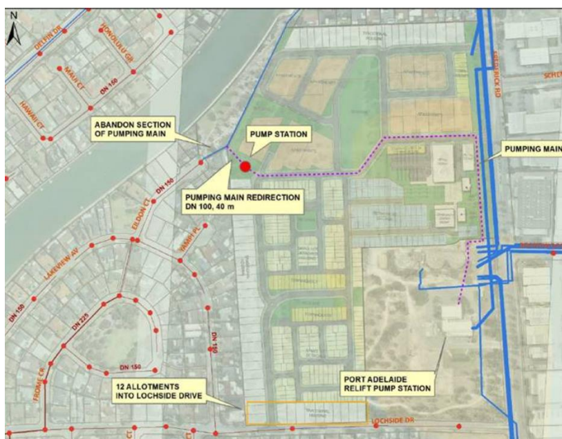
Figure 4 - SA Water waste water - markup supplied in 2017 for previous development concept plan (approximately 1,100 dwellings compared to current proposal of 570)
