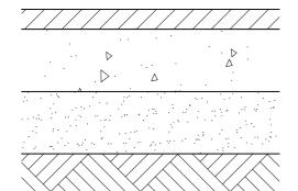
40mm AC10M (C320) WEARING COURSE 150mm PM1/20 QUARRIED PAVEMENT MATERIAL COMPACTED TO 98% MAXIMUM MODIFIED DRY DENSITY (MMDD)
