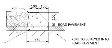
CONCRETE: CLASS N25 MINIMUM COMPRESSIVE STRENGTH 25 MPa WITH 14mm AGGREGATE
