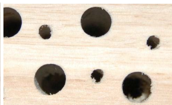
Burrows with burrs (left) will not be used by the bees. Using sharp drill bits ensures holes are smooth (right; Photos: Megan Halcroft)
